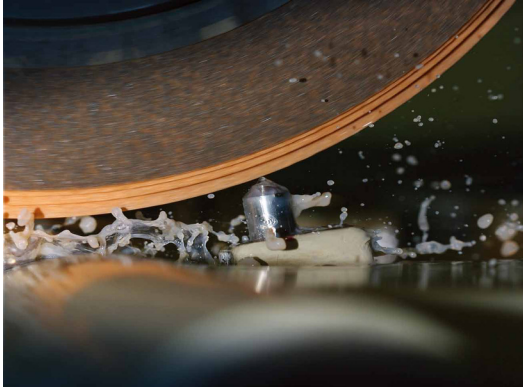
Stationary diamond dresser in contact with the grinding wheel
