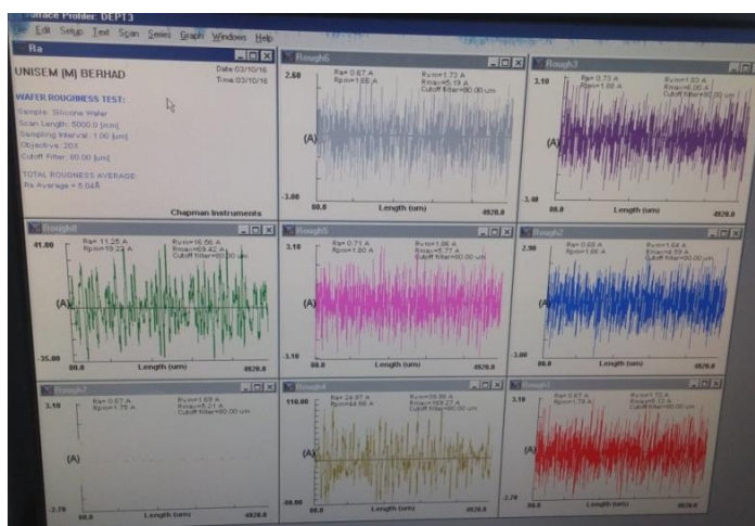
Original field measurement display from Q219 with individual profiles and unchanged measurement information.
