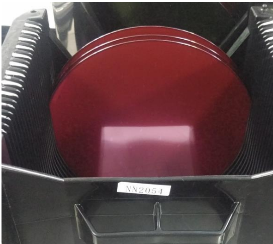
Silicon wafer in the DP process for 8 and 12 inches from Q219.
