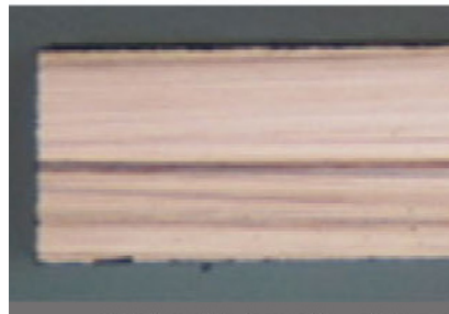
New bond: side and back chipping.
