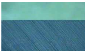
Edge image X40: wafer thickness 90 μm after rough grinding, #600 RSL.
