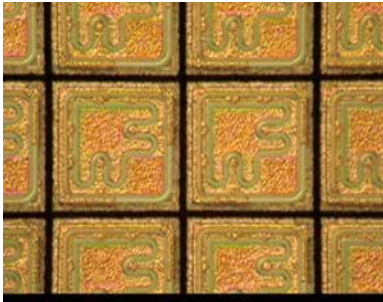
Cut image showing top-side chipping: Top Chipping.
