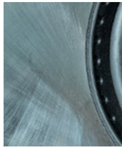
Surface detail after grinding with a grinding wheel.
