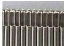
Needle tips after ECG grinding: burr-free comparison image.
