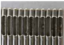
Needle tips after conventional grinding: burrs in the comparison image.
