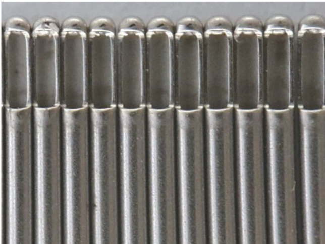
Burr-free needle tips in the illustrated ECG comparison.
