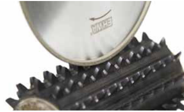
Hob-grinding application example.
