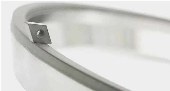
Cutting insert during peripheral grinding
