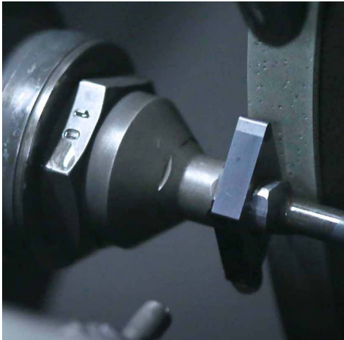
Peripheral grinding of a cutting insert
