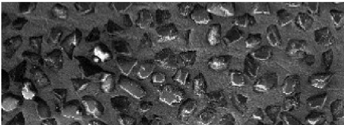
Structure image of the slotted electroplated wheel.
