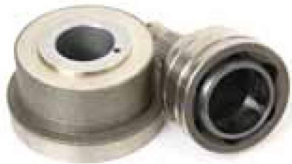
Dressers for the outer diameter of the outer race.
