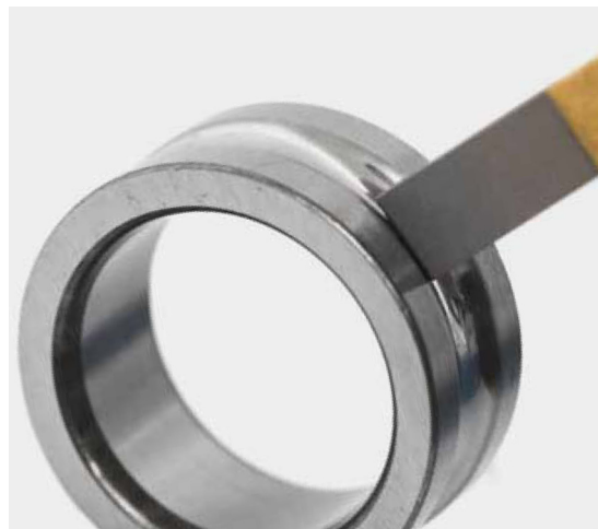
Honing stone in contact with a bearing ring
