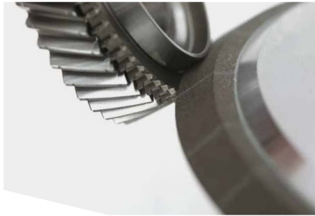
CBN grinding wheel and transmission component in angular grinding.
