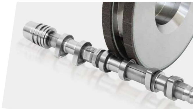
Camshaft and grinding wheel in the machining arrangement.
