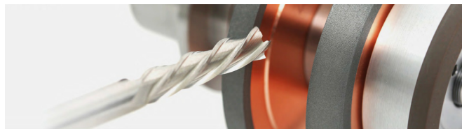
Tool and grinding wheel during flute grinding
