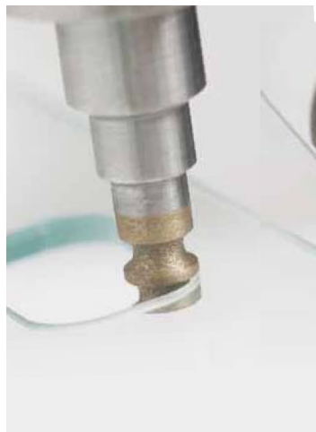
Metal-bond tool for glass-hole grinding
