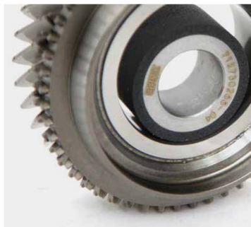
CBN internal-grinding tools and a transmission component.
