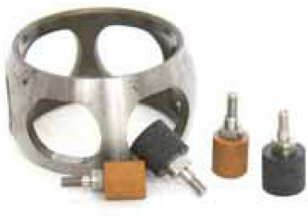
Cage and tools for cage-window grinding.
