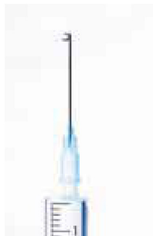
Needle workpiece made from SUS/SUS304
