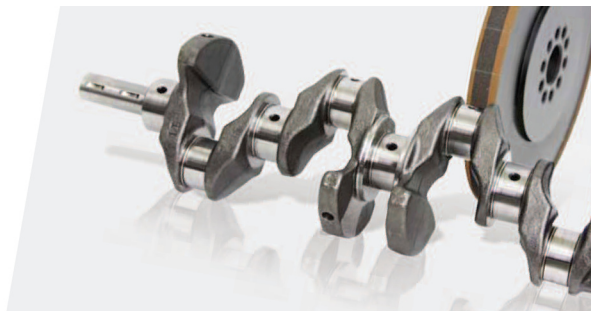
Crankshaft and grinding wheel in the machining arrangement.
