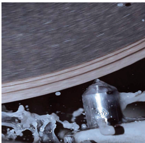
Stationary diamond dressing with coolant
