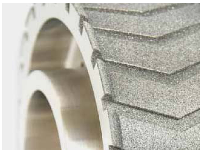
Profiled layer of the brake-pad wheel
