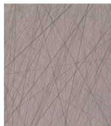
Comparison surface after lapping: copper-resin, 50 \times .
