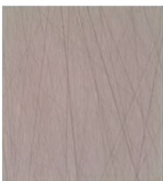
Surface after lapping: iron-resin, 50 \times .
