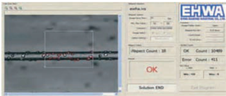
Inline inspection and real-time counting during diamond-wire production.
