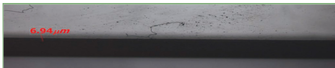
Glass edge after polyurethane polishing: local measurement marks are retained.
