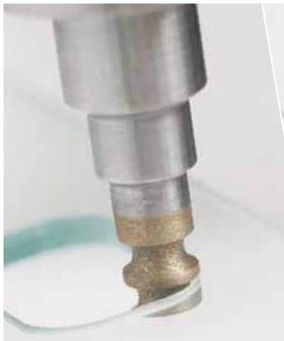
Metal-bond tool during glass-hole grinding.
