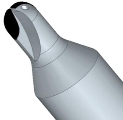
PCBN ball endmill in normal form.
