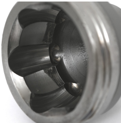
Machined raceways inside the joint housing.
