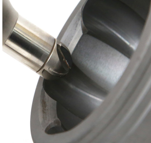
Machining an internal joint contour.
