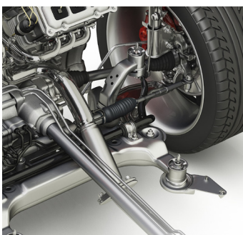
CV joint in the front-axle area.
