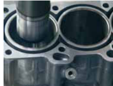
Cast-iron cylinder block: Component and machining view.
