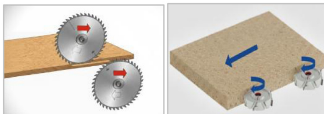
A/T cutter in edge preparation.
