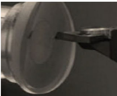
Single-crystal diamond cutting tools: Component and machining view.
