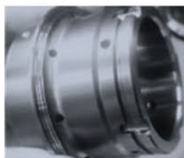
PCBN grades: steel and cast iron: Component and machining view.
