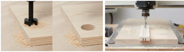
Drilling wood-based panels.
