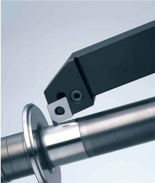
Turning tools: Component and machining view.
