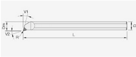
BS type: isolated dimension scheme.
