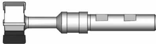
Ophthalmic lenses: edge machining: Tool view.
