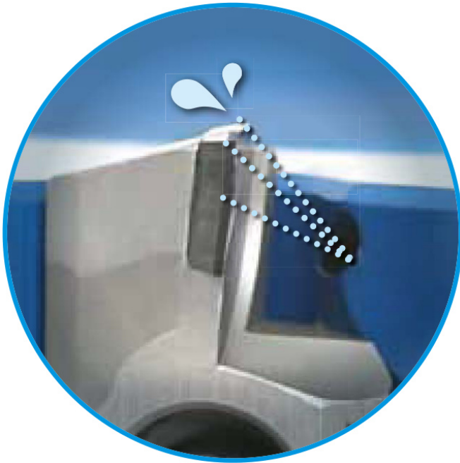
CF: cutter with directed chip and coolant flow: Component and machining view.
