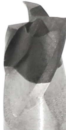
Enlarged PCD cutting edge of the highlighted small tool.
