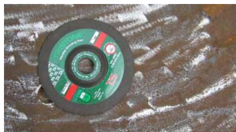
Rust removal: abrasive disc.
