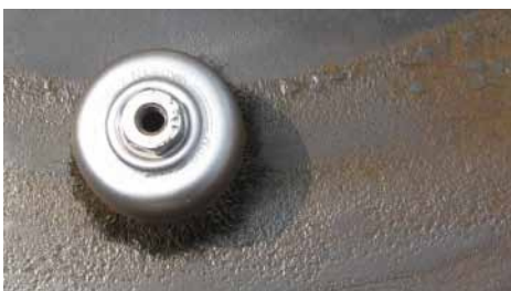
Rust removal: cup brush.
