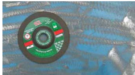
Paint removal: abrasive disc.
