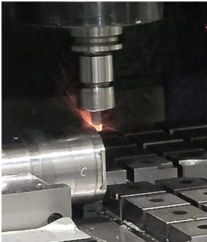
Ceramic end mill machining a component.
